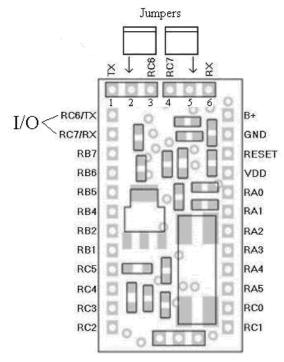
2. When RC6/TX and RC7/RX are used as a RS232 serial port place jumpers on pins 1-2 and 5-6 of the 6 pins connector.
