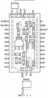
If your supply voltage ranges between 4.2V and 5.5V, connect the supply to the VDD (bypassing the onboard 5V regulator).
